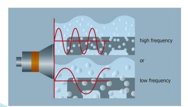
All LCT ultrasound systems can be equipped with SINGLE and DUAL frequency technology (in accordance with your wishes and requirements):
