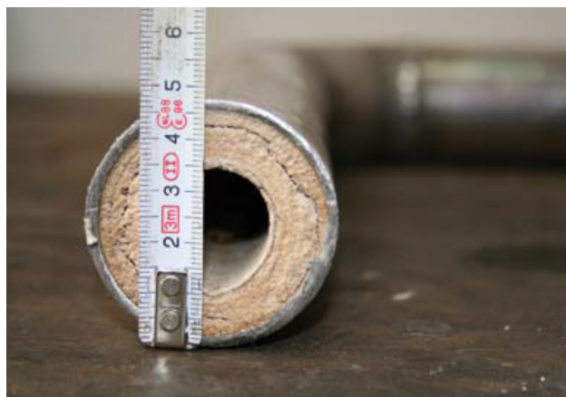
Pipe upstream of rinsing with the RWR
