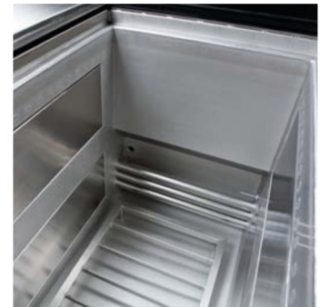
Installation view of a plate type transducer - inner side, heaters in niches
