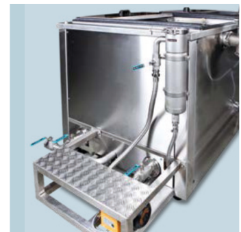
Filter circuit to increase the operating life of the cleaning medium
