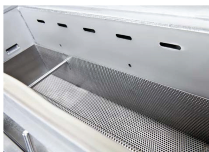
Overflow pocket, coarse filter and integrated exhausting
