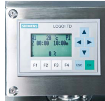
PLC control panel for ease of operation
