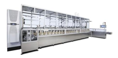
Ultrasound cleaning is often just one stage of a complete cleaning or surface finishing process. One of the core competences of LCT is customised design and construction of automatic linear systems for ultrasound cleaning, rinsing and drying or other procedures such as passivating or electrolytic polishing.
